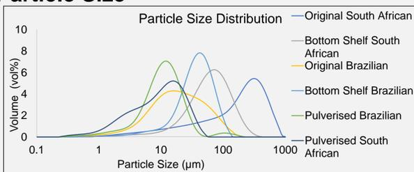
Fig. 3: Particle size distribution (PSD) of the in volumetric basis obtained from Malvern Mastersizer
