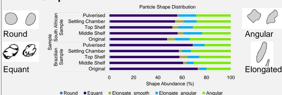
Fig. 4: Particle shape profile of the coal dust sized particles from QEMSCAN using roundness and aspect ratio.
