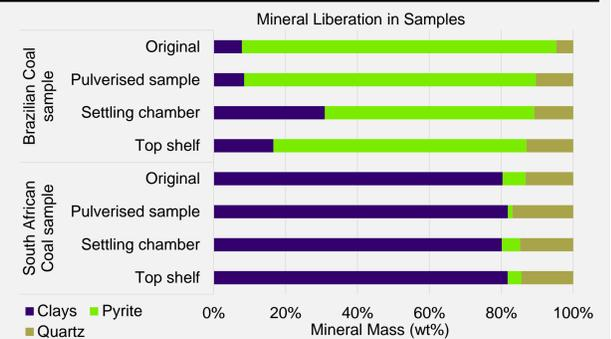
Fig. 5: Common mineral phases in dust samples
