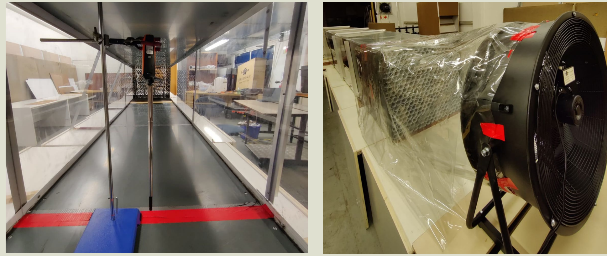
Figure 3: Retort stands holding the test anemometers inside the tunnel to measure wind speeds at different heights
