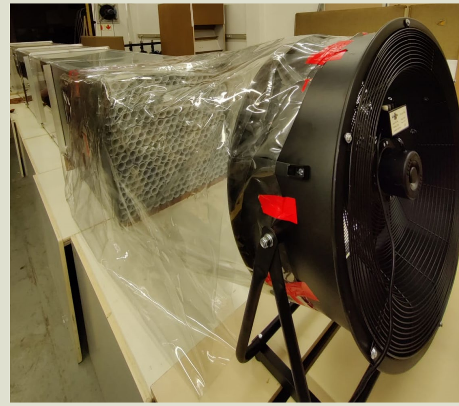
Figure 4: Fan setup at the entrance of the tunnel with channelling plastic- blowing set up
